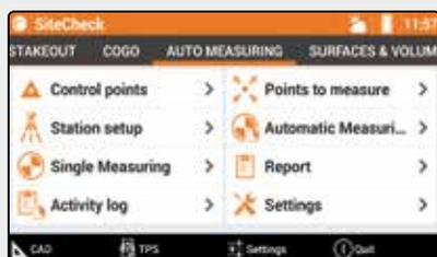
X-PAD Automeasuring is the simple, flexible, safe and economical solution for all you need to use the total station for automatic measurement and real-time checking of the movements of embankments, dams, buildings, bridges and other structures.
