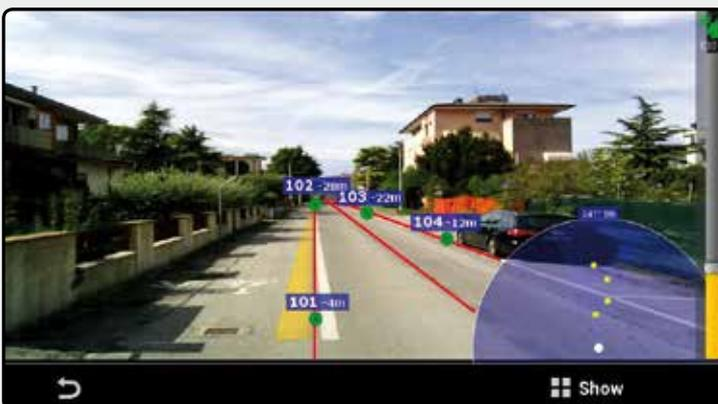
How can augmented reality be a useful tool in topographic surveys and stakeout? Point the camera to the site and you can see immediately where the points and elements are for stakeout. X-PAD will guide you in the vicinity of the point and then determine the exact location, but you can also use augmented reality to see what is not possible to see (e.g., pipes, cables and connections belowground).
