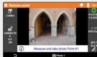
PicPoint is an innovative way of measuring points that are not directly accessible from the GPS equipment. The combination of GPS location, with the photos acquired by a calibrated camera positioned on the pole allows you to measure directly in the field but also in the office later, adding new points directly on the photo. Facades, unreachable points, edges, elements to be measured bounded by fences, etc. are all situations where PicPoint is the practical solution, fast and precise.
